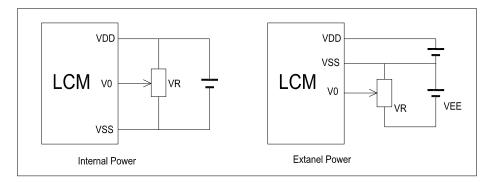
$V_{DD-V_0}$ : LCD Driving voltage VR: 10k~20k
